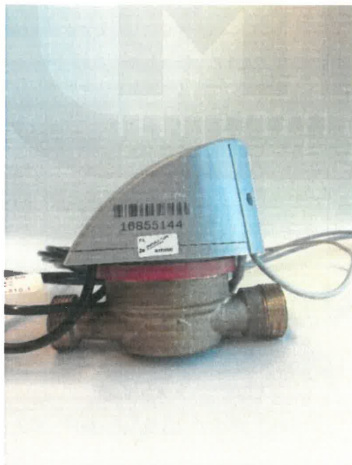
Picture 2: Sealing of compact thermal energy meters type Elf2, on side view, placement of serial number:
